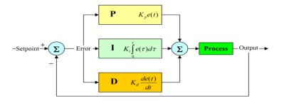
Figure 4. Block Diagram of PID Controller
