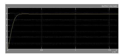
Figure 12. Output Voltage waveform of Buck Waveform using Sliding Mode Controller
