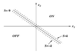
Figure 6. Sliding mode on x<sub>1</sub>-x<sub>2</sub> phase plane
