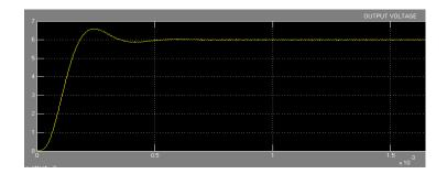
Figure 9. Output Voltage waveform of Buck Waveform using PI Controller
